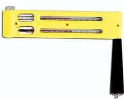
Figure 2: A whirling hygrometer. There are a number of different models and manufactures of whirling hygrometers with one of the basic models shown above. The Whirling hygrometer measures wet bulb temperature. The wet bulb temperature taken on the morning that the fruit rind temperature was taken (figure 1) was 6oC (9:40am). Since the fruit rind temperature was 3.9oC, this equates to a ( 6 - 3.9 ) 2.1oC difference. The recommended minimum difference requirement for harvesting is 3oC and therefore in these conditions harvesting should not commence.
