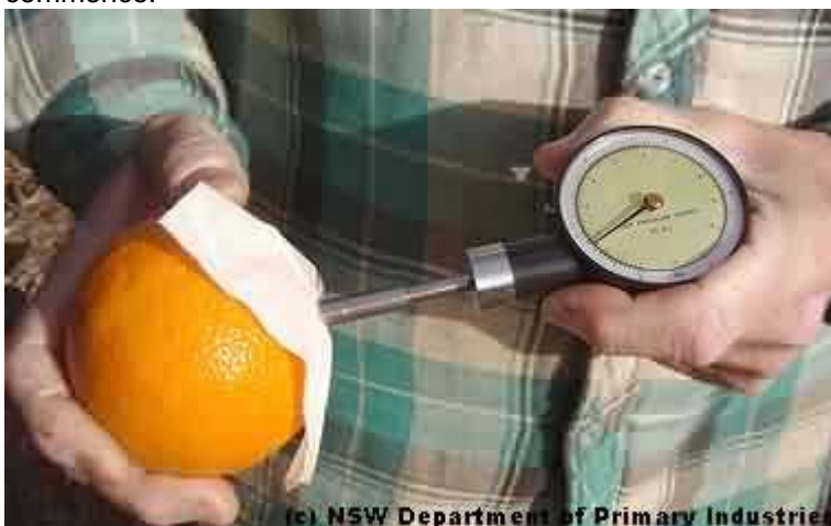
Figure 3: Rind Oil Release Pressure (RORP) Test : A penetrometer being used to check the rind oil release pressure for a Washington Navel. Note that the wet bulb test must first pass before this test is taken.
