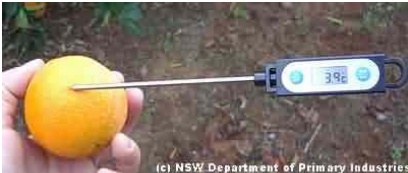
Figure 1: Rind Temperature : A digital thermometer inserted a few millimetres into the rind of a Washington Navel. Notice that the thermometer is inserted on an angle into the rind to prevent the thermometer penetrating into the pulp of the fruit.
